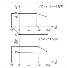
Permissible values for ambient temperature Tu at housing are dependent on the operating temperature
